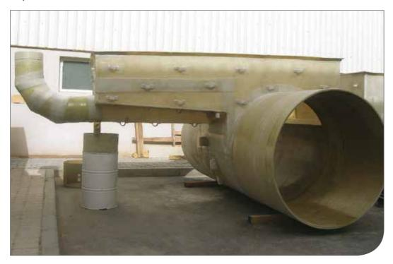
GRP Liners are basically used to protect the structure from corrosion due to the acid and gases formed during sewage metabolism. Inter Pipe Factory manhole liners are flexible composites constructed of a thermosetting chemical resistant resin, glass fiber reinforcement and additives as required. The manhole is a cylinder that can be provided with benching unit, cover slabs with a round or square opening, and the lugs fixed as per the appropriate project drawings.
